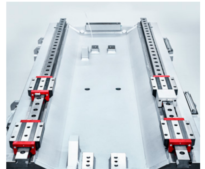
Guides for the moving column Y axis travel.
